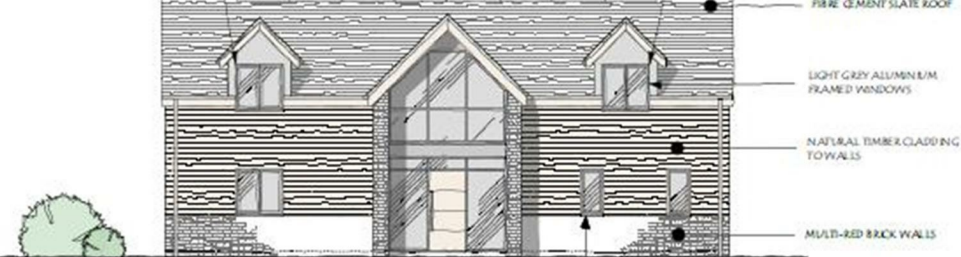
SOUTH EAST ELEVATION (FACING COURTYARD)
